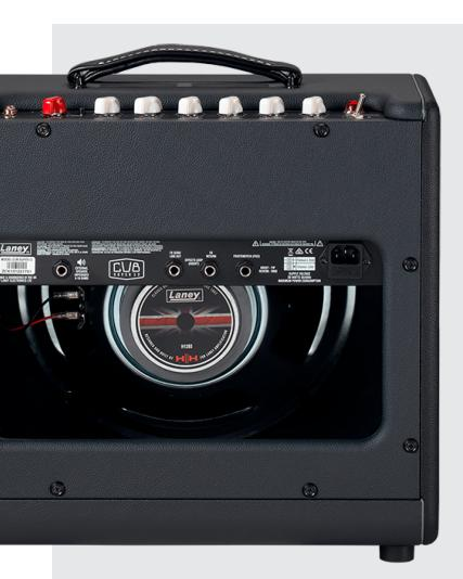
The Cub-Super12's five valves – three selected 12AX7s and a pair of EL84s – are mounted pointing forwards and can only be replaced by removing the chassis. The loudspeaker is a custom-designed HH Electronics H12-65 with a medium-weight ceramic magnet helping to keep things portable.
